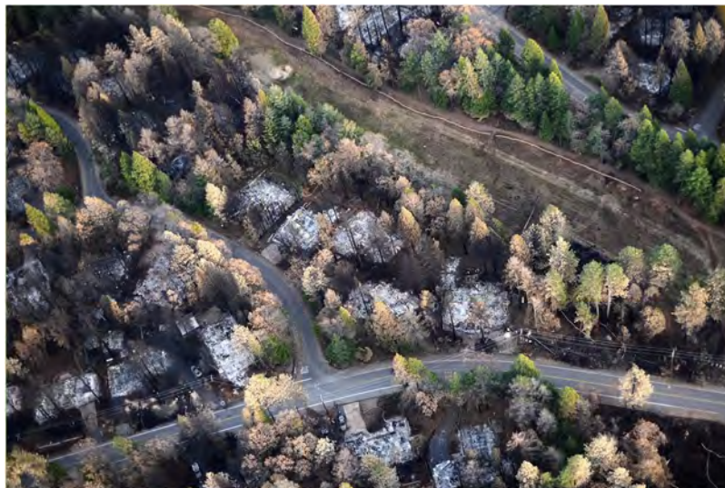
Fig. 7 Aerial image showing a portion of Magalia just NW of Paradise, illustrating a gradient of fire damage to overstory vegetation with distance from destroyed homes. At least in some areas, burning homes may have influenced the effects to overstory vegetation more so than burning overstory vegetation influenced the outcome to homes. Photo: Owen Bettis, Deer Creek Resources
