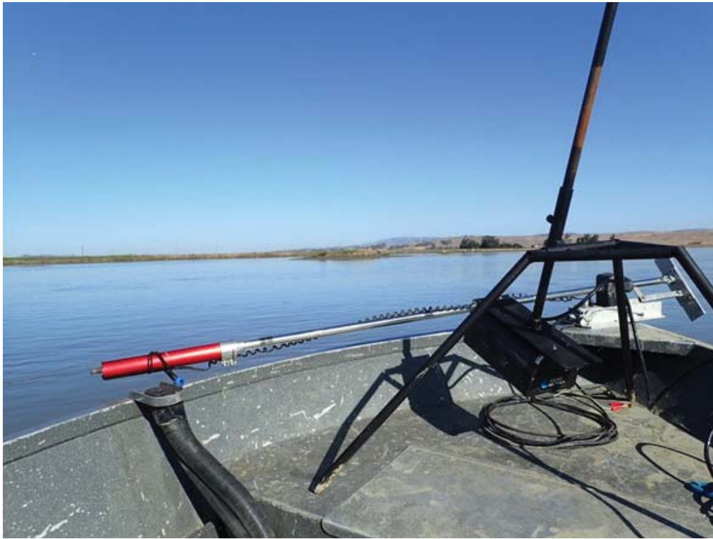
Figure G-1. ARIS camera attached to the stationary stand with transect mount attached to the boat behind.
