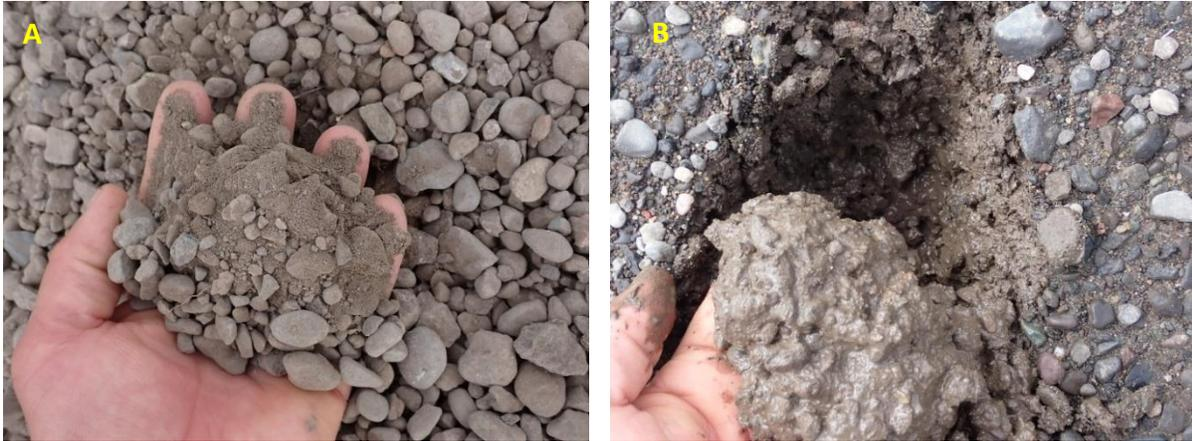
**Photograph 19. Dry and wet pea gravel with interstitial sand and mud (fines) composing gravel berms**
