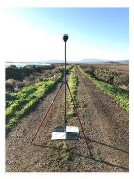
Figure 2. Typical aerial target survey.
